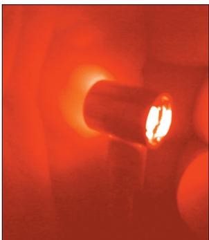
*Integrating sphere-based laser diode power meters offer accurate measurement while eliminating sensitivity to alignment.*
