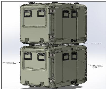
The system enclosure is divided into two halves; the 8 inch integrating sphere with the lamp, VA and detection devices are in the top half, and the supporting electronic components are rack-mounted in the bottom half. A thermally insulated ceiling/floor partition separates the two halves. Both halves contain fan-cooled heatsinks and temperature monitoring points for over-temperature protection that will shut off the system before thermal damage occurs.
