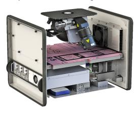
A sealed diffuser window is located at the top of the system enclosure right above the sphere's exit port to protect it from outdoor weather. The sphere illumination includes a fan-cooled HES-150 (150W), external QTH lamp with a manually adjustable variable aperture attenuator (VAM) that enters the sphere through a 5 position, 2 inch filter wheel (HFW-5-2) for color and band filtration of input energy.
