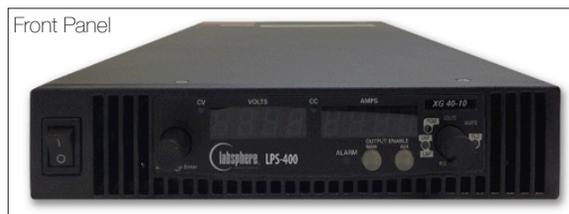
The LPS-400 unit is used with all HELIOS Lamp Assemblies in standard system configurations. The 40V/10.5A power profile will run all HIS and HES lamps below 200W and will also run the PEL-250 Plasma Lamp Assembly. Xenon lamps do not require the LPS-400 as they have an internal power unit.
