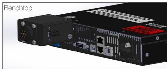
**Benchtop Option:** Unit attached to the back of the standard LPS-400 or 850 that converts from terminal outputs to our standard HIS or HES cable adapter. Fan power inputs (from wall wort) and a selector switch that enable the fan power are included. Also includes wall power supply with radio jack for 30W/12V/2.5A power to the fan (Part#1035-2). The wall power supply is required for the HES lamps (integral fan) but not for the HIS lamps.
