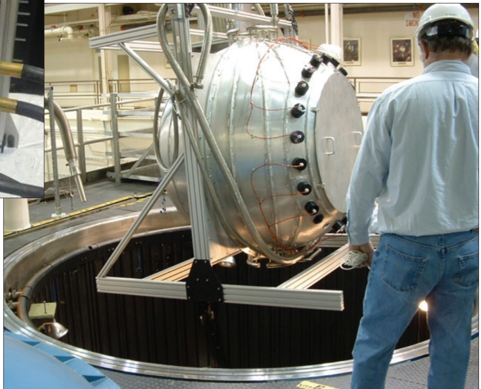
Vacuum, 1.5 m LN 2 Cooled 8 kW Absolute Uniform Source Descending into NASA 3 m TV Chamber
