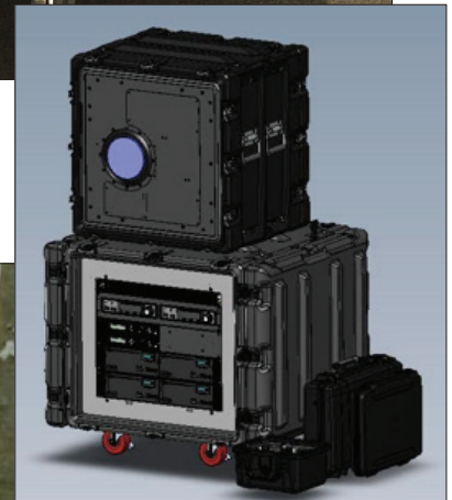
Ruggedized Hyperspectral Calibration Source for Hangar and Runway Deployment
