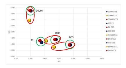
The red ovals show the tunable sources and SSL sources that are intended to represent the standard illuminant for the same CCT. Even though the CCTs are similar, the ratios for the solid state phosphor sources do not represent the desired ambient illuminants.
