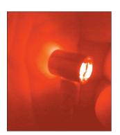
Integrating sphere-based laser diode power meters offer accurate measurement while eliminating sensitivity to alignment.
