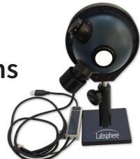
The systems provide options for laser power measurement over the 350 to 1700 nm wavelength region for optical powers ranging from nW to tens of watts. The system's calibrations are traceable to the National Institute of Standards and Technology (NIST).
