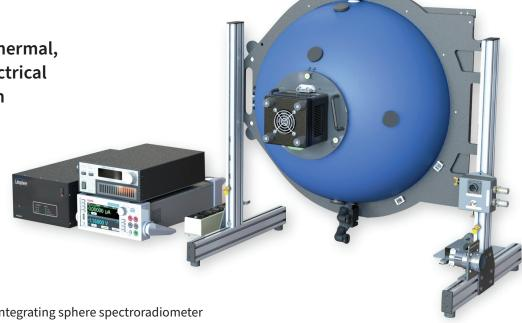
The illumiaPro3 is an integrating sphere spectroradiometer designed specifically for the testing and characterization of high-power LEDs. With Labsphere's powerful Integral® software control, it's a turnkey solution with embedded routines that guide the user through industry test methods and standards, yet completely flexible for research, development, and quality inspection.
